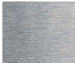
Surface finish: machined, Ra 0.8 \mu\text{m}
