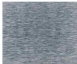
Surface finish: fine-machined, and grinded, Ra 0.2 \mu\text{m}
