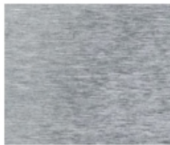
Surface finish: fine-machined, and grinded, Ra 0.4 \mu\text{m}
