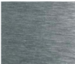
Surface finish: machined, Ra 1.2 \mu\text{m}
